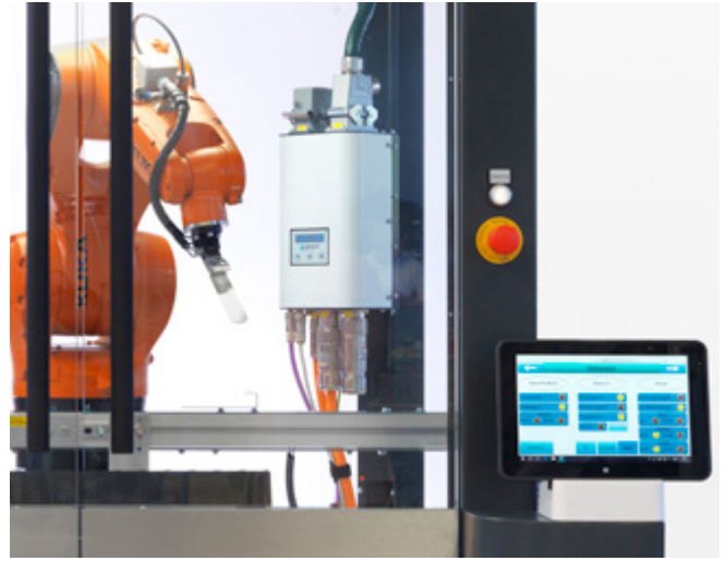
KUKA robot, Plamatreat PCU and control panel
